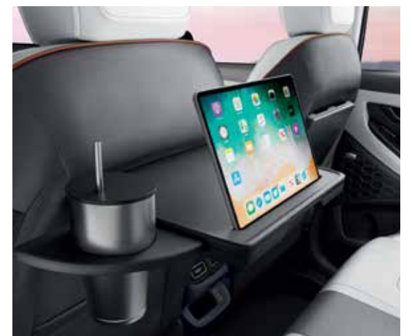
Front row seat back table with IT device holder & retractable cup holder
